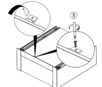
Installation of the front panel with front rail for H167 & H199 inset drawers
