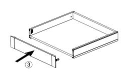
Installation of the front panel with heighten panel for H167 & H199 inset drawers
